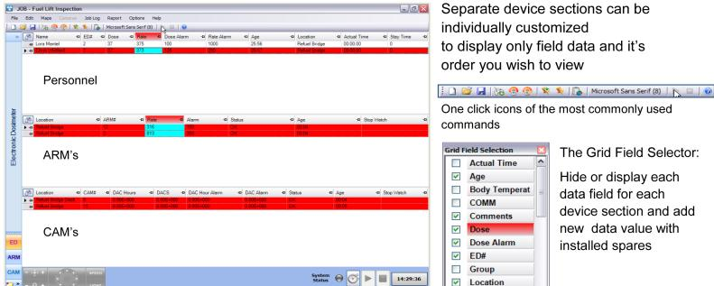
Separate device sections can be individually customized to display only field data and it's order you wish to view
